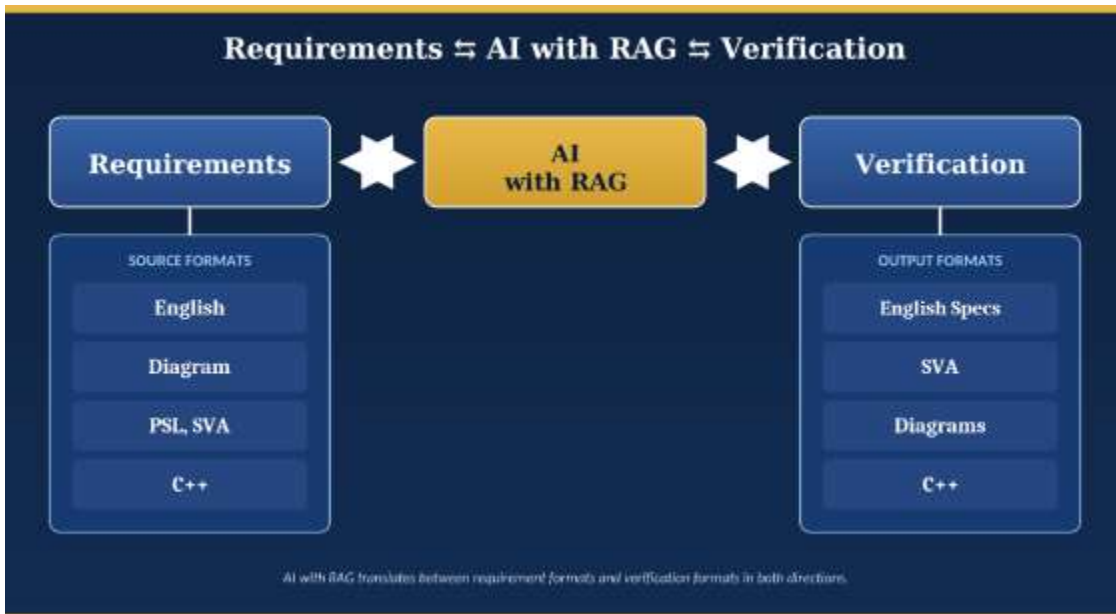
Figure 2 — AI with RAG sits between requirements and verification and translates in both directions: English, diagrams, PSL/SVA, and C++ on one side; English specs, SVA, diagrams, and C++ on the other.
